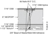
Continuous Perimeter Support by Other Required. Minimum Bearing is 3". Screw Panels @ 6" O.C. Along Perimeter.
