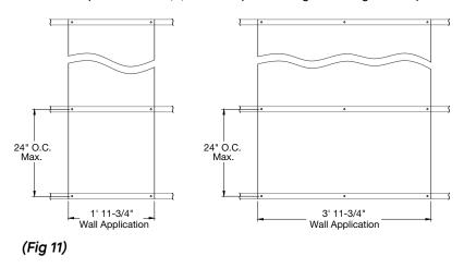
**NOTE:** Short side of panel (panel width) is undersized at 23-3/4" or 47-3/4", while long side of the panel is 48" or 96".
