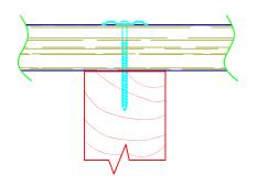
ONE ROW OF SCREWS IS REQUIRED AT INTERMEDIATE SUPPORT.
