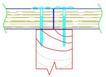
TECTUM I DECK USES DEKFAST #14 SCREWS WITH 2" WASHER. MINIMUM LENGTH IS ONE INCH LONGER THAN PANEL THICKNESS. 1½" PENETRATION PREFERRED.
