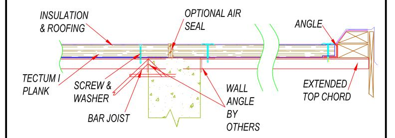
NOTE: PANEL CAN BE SCREWED TO MASONRY WALL INSTEAD OF ANGLE. IT IS NOT PRACTICAL TO SCREW THOUGH A PLATE INTO MASONRY. SEAL REQUIRED FOR SWIMMING POOLS, ICE RINKS, ETC.
