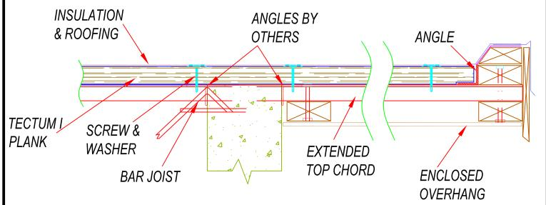
NOTE: PANEL CAN BE SCREWED TO MASONRY WALL INSTEAD OF ANGLE. IT IS NOT PRACTICAL TO SCREW THROUGH A PLATE INTO MASONRY.
